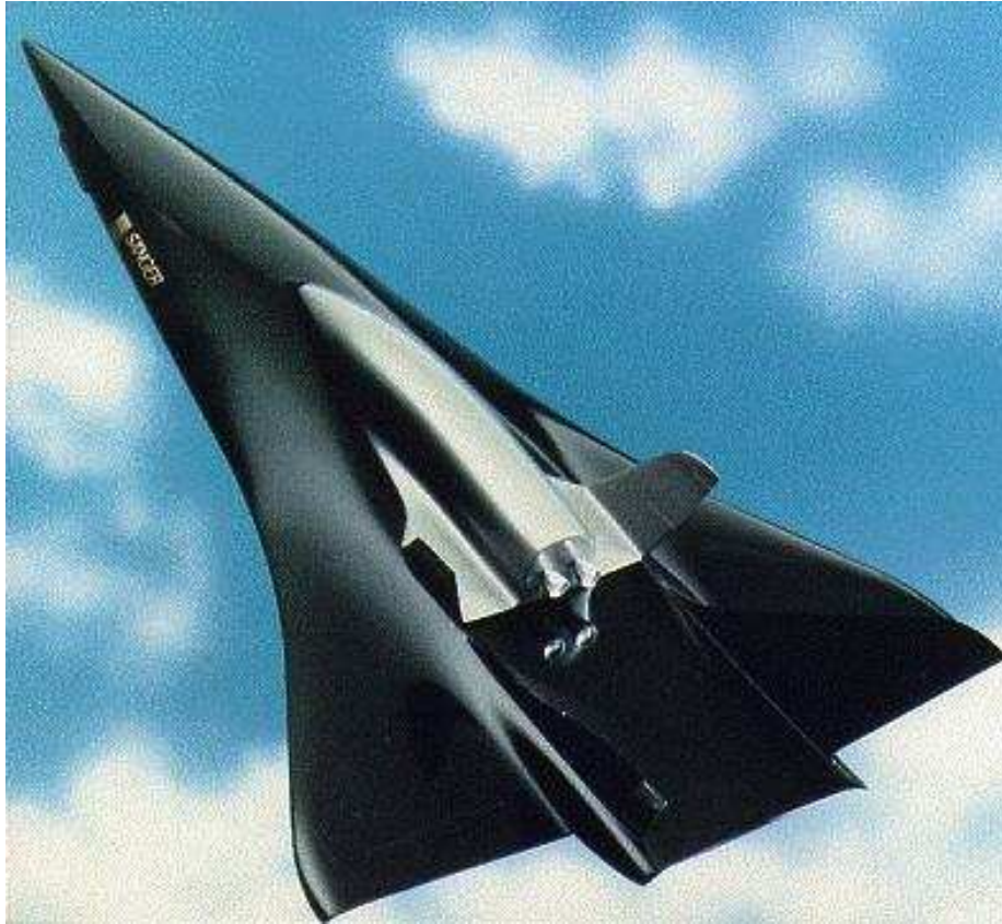
FIGURE 1. A detailed model of the lower stage of the German two-stage-to-orbit concept Sänger II [1], [5] provides the model for a hypersonic passenger aircraft, which gave the motivation for the “hypersonic car problem” investigated in [3], [4].
