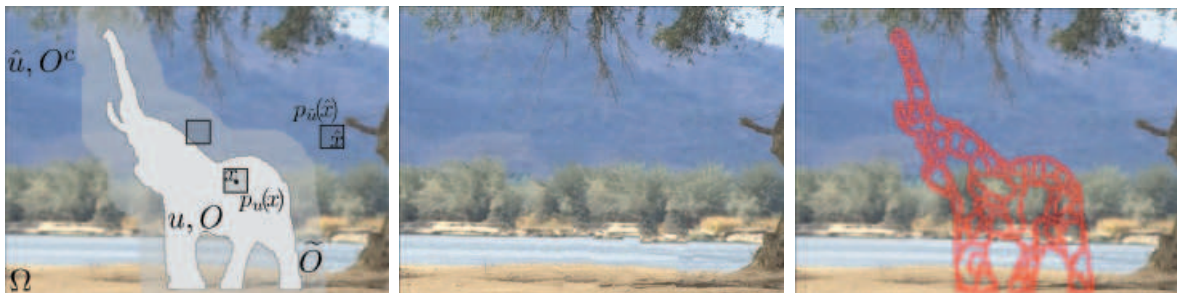
FIGURE 1. Inpainting problem. Left: on a rectangular image domain \Omega , missing data u in a region O has to be reconstructed using the available image \hat{u} over O^c := \Omega \setminus O . The set of centers of incomplete patches is \tilde{O} := O + \Omega_p , being the latter the patch domain. The center image shows a completion found with one of the one of the schemes derived from the framework. Right: the resulting completion is a patch-work built by copying arbitrarily shaped regions from O^c . The red curves show the boundaries between the copied regions.
