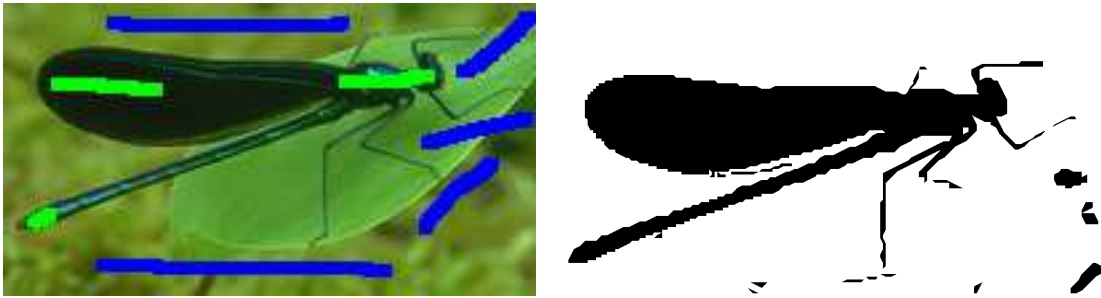
FIGURE 2. User-labeled input image and globally optimal curvature regularized segmentation computed via linear programming relaxation. Source:[6].
