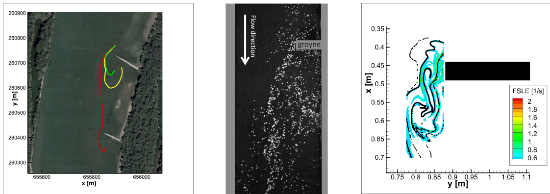
FIGURE 1. Left: Trajectories of three surface buoys in River Danube in the vicinity of a groyne field. Middle: Laboratory setup with a single groyne and the floating particles used for the PTV- measurements. Right: FSLE ridges (colored) and the largest flushing times (black) at t = 0 s. The groyne is marked as a black rectangle.
