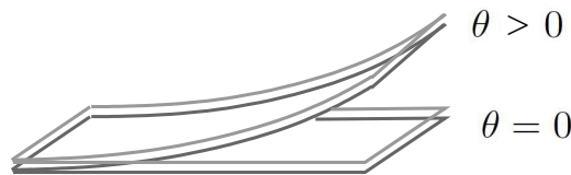
FIGURE 1. Bending of a bilayer sheet due to a mismatch of material responses to, e.g., temperature.
