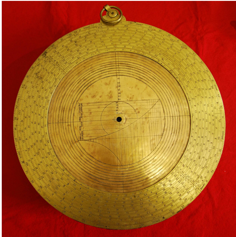
FIGURE 1. Albion ( \phi = 325 mm), made in central Europe in the 15th century, following the instructions in Richard of Wallingford, Tractatus Albionis (1326). Rome, Museo Astronomico e Copernicano
