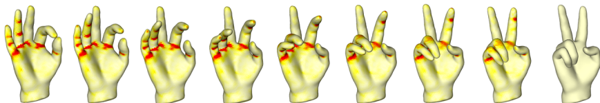
Figure 2: Accumulating small variations to generate a complex motion or large deformation. Here, the color encodes a measure of local variations (red means high). The accumulated local dissimilarity measure between consecutive shapes then leads to a global distance measure between the two boundary shapes (leftmost and rightmost hand).
