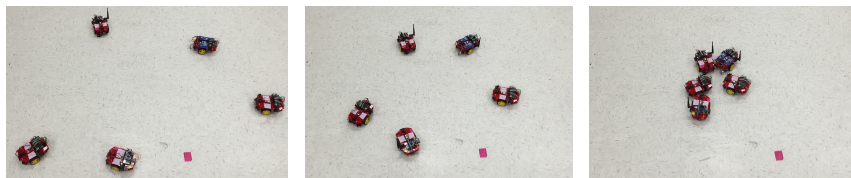
Figure 3: Five robots meet. They all aim towards the centers of their neighborhoods.
