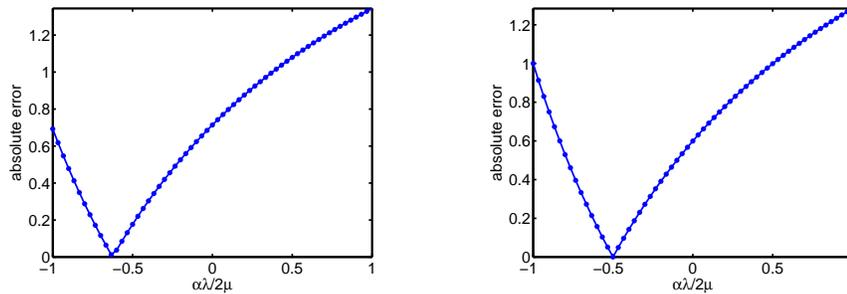
FIGURE 2. Error of the vertical tip displacement at  $A$  versus  $\frac{\alpha\lambda}{2\mu} \in [-1, 1]$ , Case IV (left) and Case I (right)
