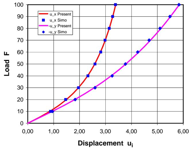
FIGURE 2. Load versus deflection for the hemispherical shell
