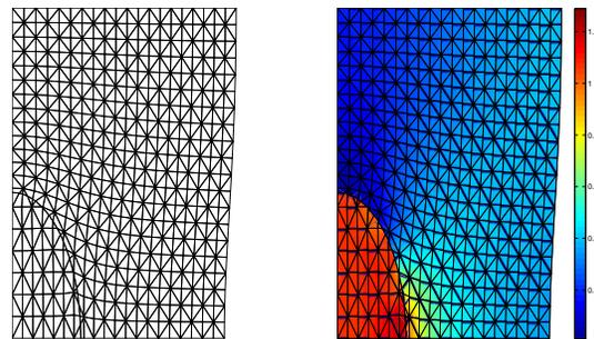
FIGURE 3. deformation and strain in a plate with soft circular inclusion
