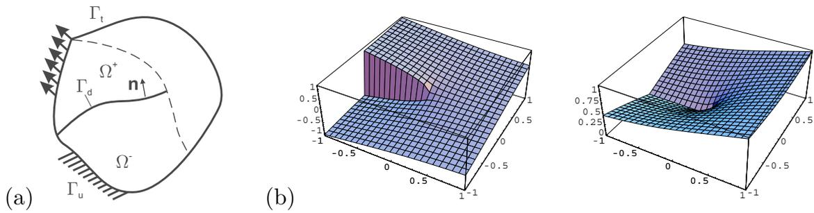
FIGURE 1. (a) Continuous body with discontinuity line; (b) Crack-tip base functions  $F_1$  and  $F_2$
