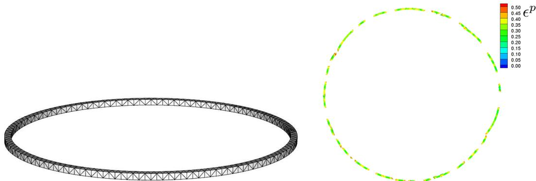
FIGURE 1. Finite element mesh for the U-6%Nb ring and fragmentation of the ring at  $90\mu\text{s}$ .
