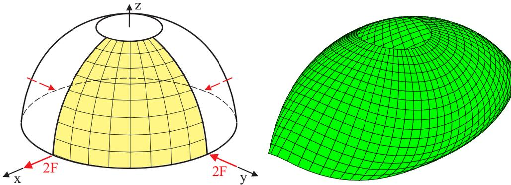
FIGURE 1. Hemispherical shell and deformed mesh for  $F=100$
