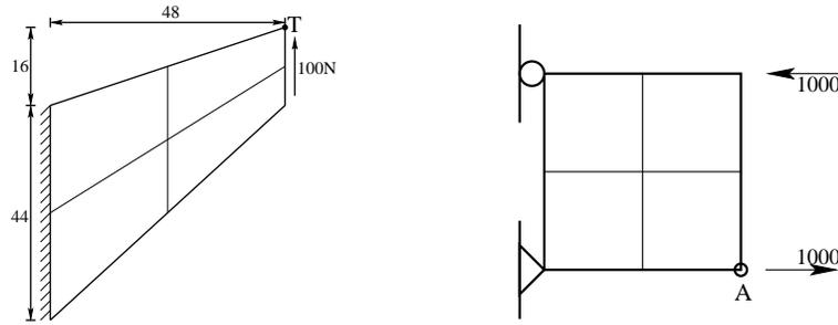
FIGURE 1. (a) Cook's membrane problem with initial triangulation; (b) the square beam problem with a mesh of four squares
