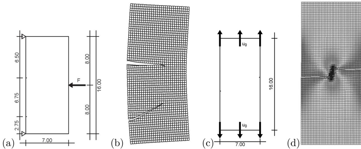
FIGURE 2. Geometries and crack-paths in a three-point bending test and a tension test.
