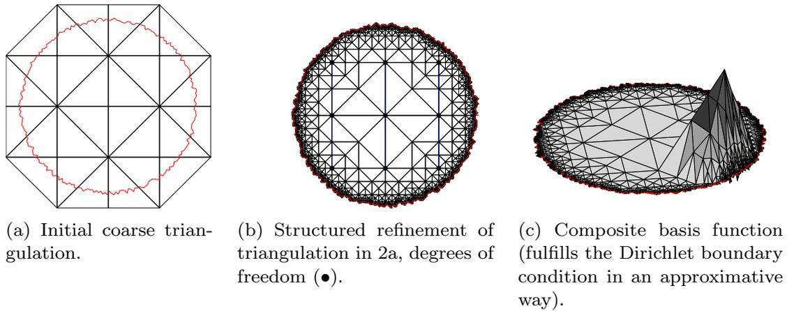
FIGURE 2. Structured overlapping triangulation of a two dimensional domain with a rough boundary and composite finite element basis function.
