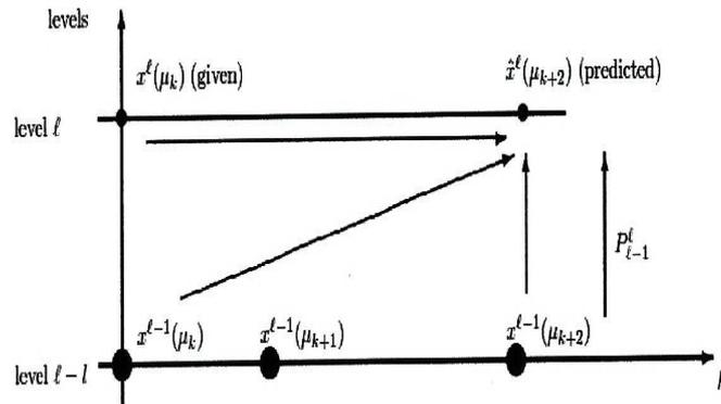
FIGURE 1. Two-level predictor-corrector scheme
