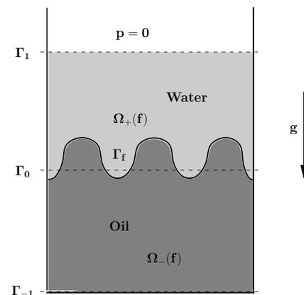
The laterals and the bottom of the cell are assumed to be impermeable and the pressure is normalized to be 0 on the boundary component  $\Gamma_1$ . It is very common in literature to presuppose that the fluids are separated by a sharp interface which moves along with the fluids.
