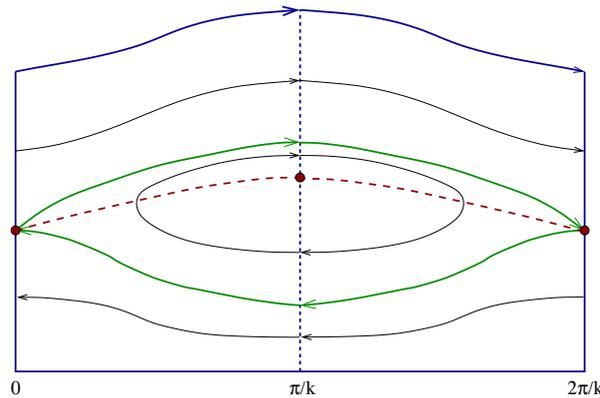
It is also possible to obtain a qualitative picture of the particle trajectories in the original physical frame. If the wave speed is chosen so that the horizontal velocity component  $u$  has zero average on the bed the following picture emerges.
