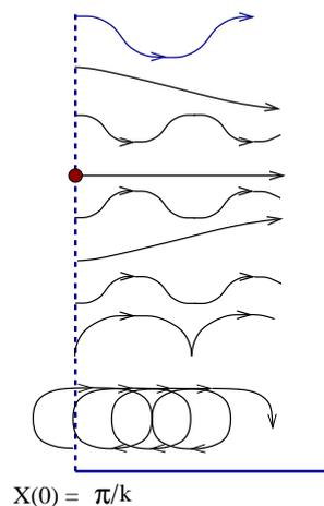
The behaviour near the bottom, where the particles move in almost closed ellipses with a small forward drift, agrees with a recent investigation of the particle motion in irrotational Stokes waves [1]. However, farther up in the fluid there is no backward motion at all, in contrast to the irrotational case.
