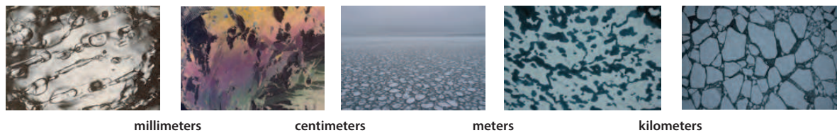
FIGURE 1. Multiscale structure of sea ice. From left to right: Sub–millimeter scale brine inclusions form the porous microstructure of sea ice [22]. When the temperature exceeds a critical value, the brine phase percolates enabling fluid flow, which mediates a broad range of key climatological and biological processes. The centimeter scale polycrystalline structure of sea ice [1] helps determine its strength and fluid flow properties. Decimeter to meter scale pancakes forming in a wave field in the Southern Ocean (Golden). Wave–ice interactions have historically been important in the Southern Ocean, and have become increasingly significant in the Arctic Ocean with receding sea ice and larger fetch. Meter to kilometer scale melt ponds on the surface of Arctic sea ice in late spring and summer (Perovich) determine the albedo of sea ice, a key parameter in climate modeling. Kilometer scale (and smaller) floes in the Arctic sea ice pack (Perovich) exhibit local diffusion in interacting with other floes and are advected in larger scale wind and current fields.
