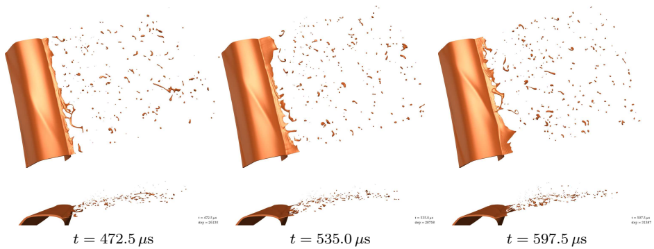
FIGURE 1. Time- and spatially-varying inflow film thickness, high mesh resolution, and shaping air currents simulating nozzle inlets. Three-dimensional model results using a high-resolution computational mesh together with accurate smooth cup geometry. Two viewpoints at the same time frame are given: a top-down perspective and a side-on view to show the vertical drifting of the shedding droplets, being pushed upwards by the shaping air currents. The liquid surface is colored copper, with the bell cup situated beneath.
