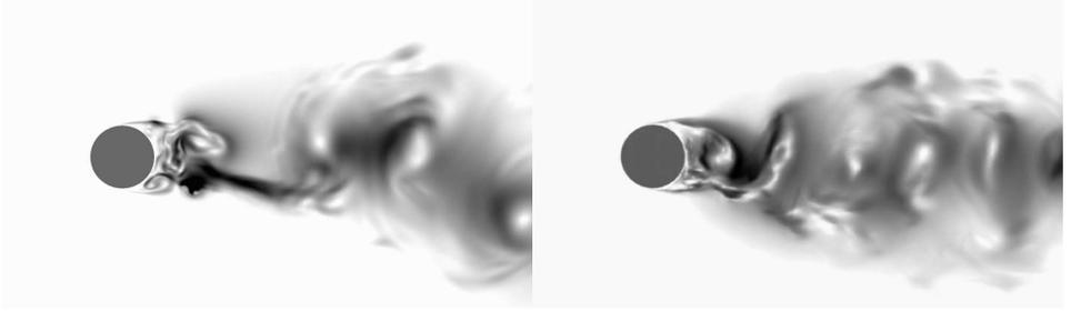
FIGURE 1. Two snapshots of the turbulence strength in the Kármán vortex street: from Large eddy simulation [15] (left), and generated by DCGAN [5] (right).
